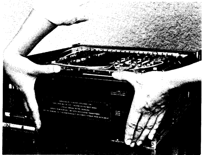
Figure 8-3-3. Power Supply Removal
